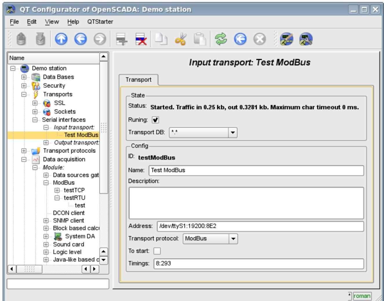
Fig.1. Configuration dialog of the incoming serial interface.
