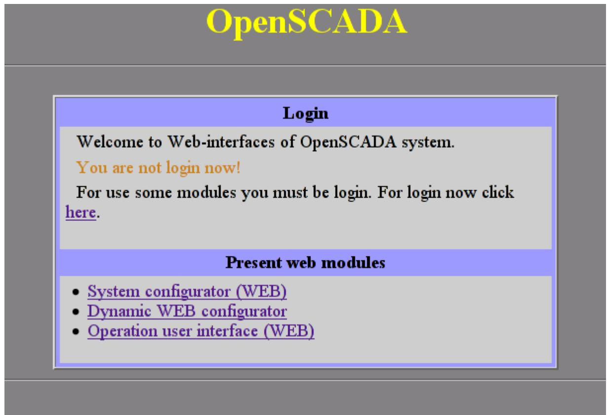
Fig.1. Dialog of the choice of WWW-interface module.
