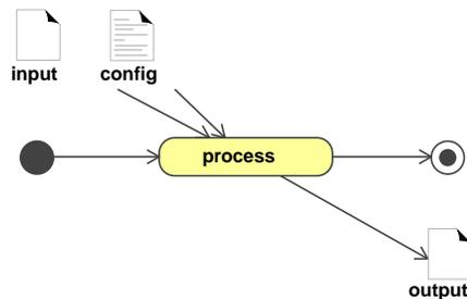
The requirement that processors can be composed into a pipeline has some important consequences for its design. The process method takes an `ir` argument, which it will operate on, and then return. It is this `ir` that forms the backbone of the pipeline, as it is passed along from one processor to the next. Additionally, parameters may be passed to the processor, such as input and output.
