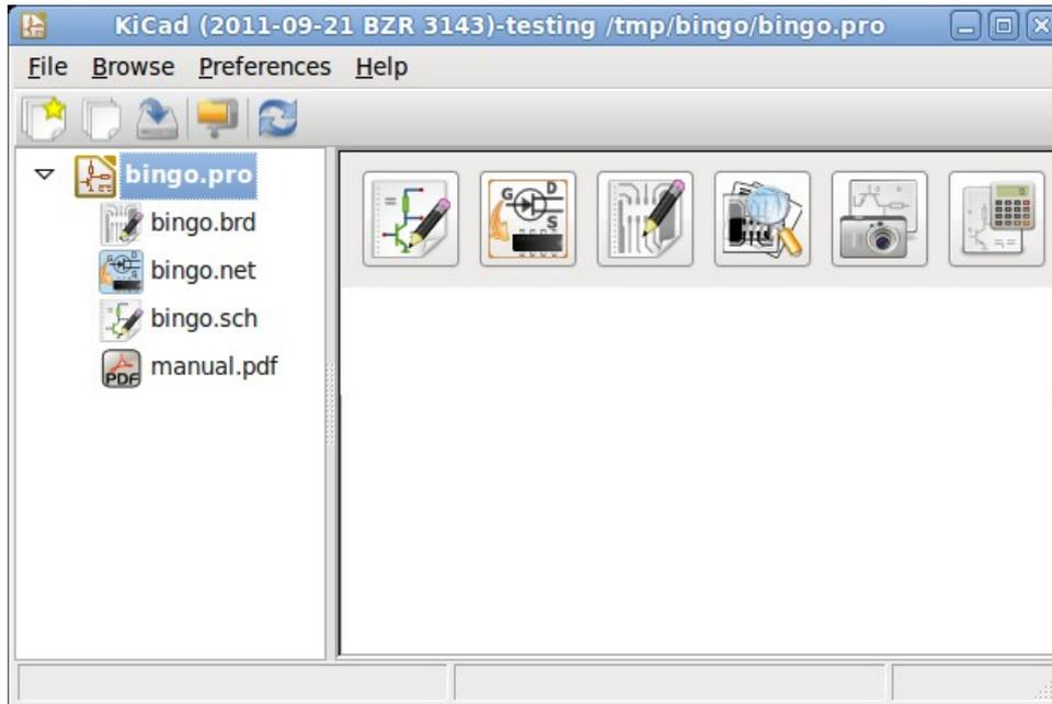
The main KiCad window is composed of a project tree view, a launch pane containing buttons used to run the various software tools, and a message window. The menu and the toolbar can be used to create, read and save project files.
