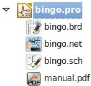
Double-clicking on the Eeschema icons runs the schematic editor which in this case will open the file bingo.sch.
