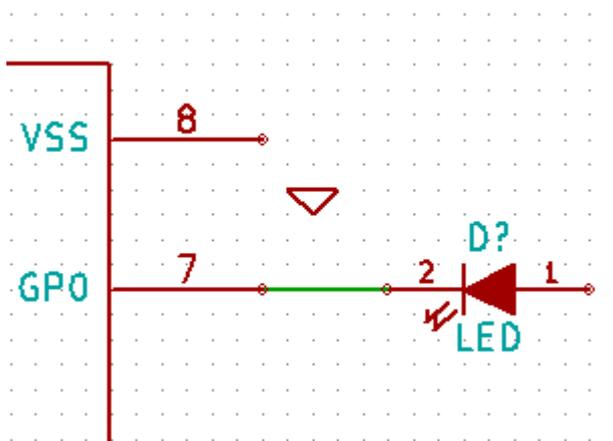
83. Repeat this process to wire up the other components as below. To terminate a wire that isn't connected to anything, double-click the left mouse button. When wiring up the VCC and GND symbols, the wire should touch the bottom of the VCC symbol and in the middle top of the GND symbol.
