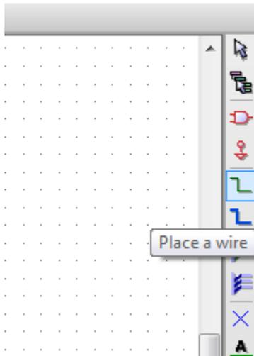
82. Left click on the little circle on the end of pin 7 of the microcontroller and then on the little circle on pin two of the LED. Alternatively, you can use the **W** key instead of a mouse click. Note: sometimes, a double-click is necessary to end a wire. In such a case the **W** cannot terminate a wire. When click/**W** while not at a small circle, then a bend is inserted.
