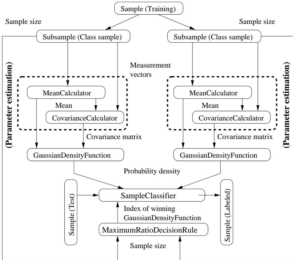
Figure 5.7: Bayesian plug-in classifier for two Gaussian classes.
