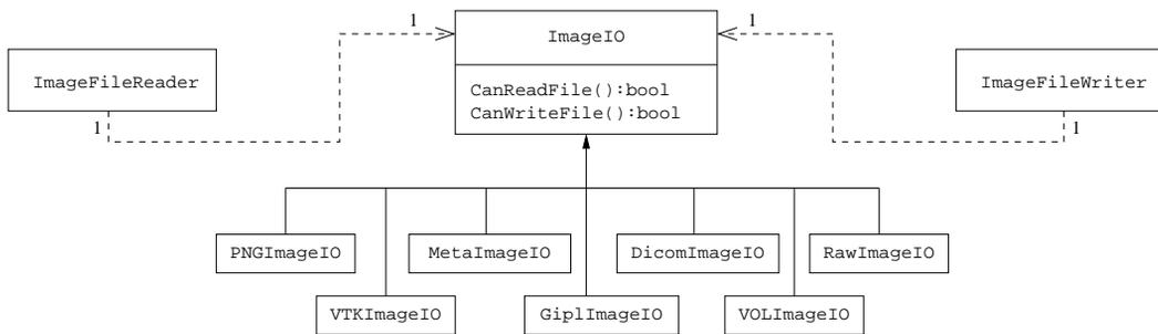
Figure 1.1: Collaboration diagram of the ImageIO classes.
