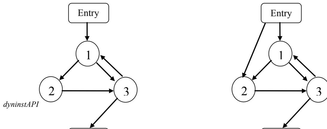
Figure (a) above shows a natural loop, where block 1 represents the single entry and block 1 is the head of the loop. Block 1 dominates block 2 and block 3. Figure (b) above shows an irreducible loop, where block 1 and block 2 are the entries of the loop. Neither block 1 nor block 2 dominates block 3.
