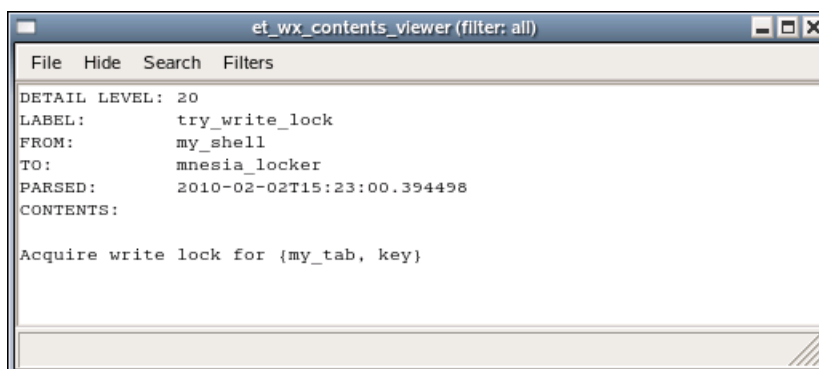
Figure 3.3: Details of a write lock message
